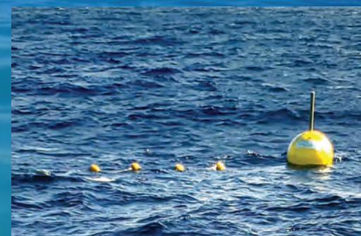
Echosounder buoy tethered to a FAD off Guam. Photo: Jaime Bass, Guam DAWR
