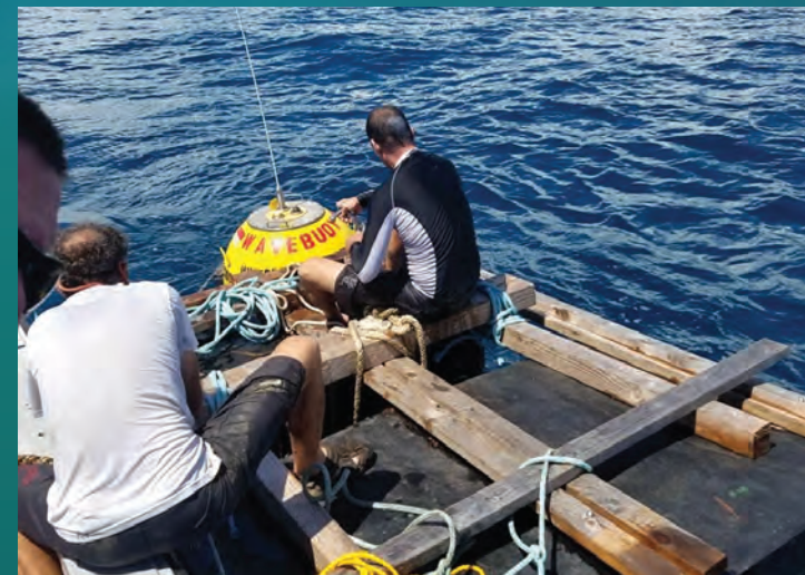
Although not new, wave buoys play an important role in fishing safety. They transmit critical weather information fishermen need to plan their day, such as wave height, wave length and water temperature. Photo: Jason Miller and Pacific Islands Ocean Observing System
